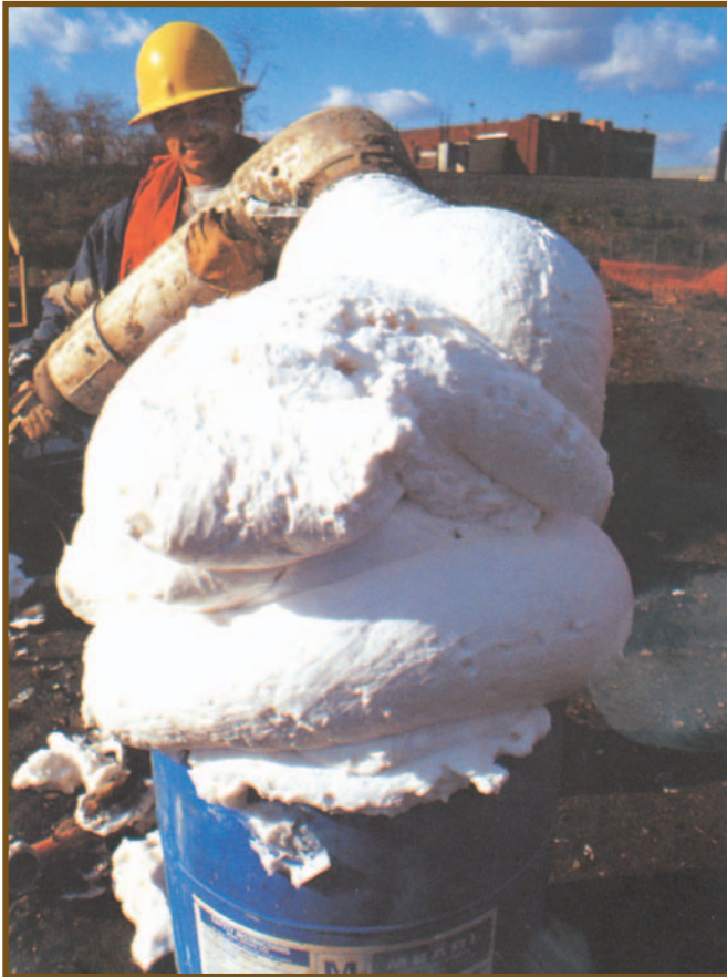
Geofoam SP is an engineered, aqueous concentrate specially formulated to yield a stable, voluminous, micro-bubbled foam. When blended with cementitious slurry, the foam enables the production of pervious cellular lightweight concrete (PCLWC), a permeable, open-cell, lightweight concrete able to stabilize soil without disturbing or redirecting natural water flow.
