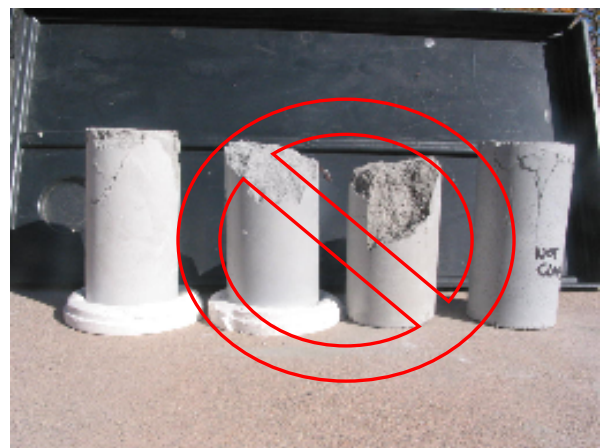
Figure 2: Incorrect cylinder breaks
