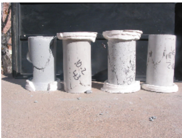
Figure 1: Correct cylinder breaks
